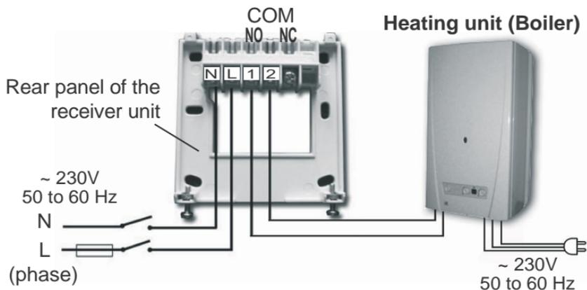
230 V mains voltage should be supplied to the receiver unit. We recommend using a fixed cable instead of a fork type connection for mains connection to avoid any unintentional de-energization of the device. We propose to connect the neutral wire of the network to point **N**, while the phase conductor to point **L**. We propose to interpose a switch so that the receiver unit can be de-energized if required.
