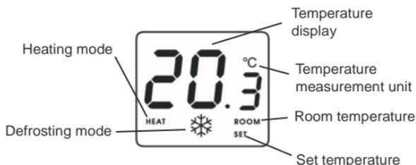
This wireless (radio-frequency) thermostat can also be extended with the receiver RX socket if needed, with which the thermostat is able to control boilers or any other electrical devices operating on 230 V (50Hz; max. 10A) (e.g. fan heaters, pumps, zone valves, etc.) according to the room temperature. (For more information please consult our website).
