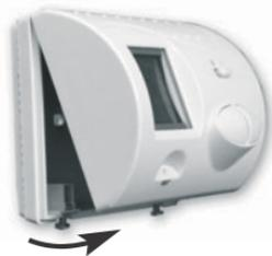
The battery compartment is in the inner side of the front panel of the housing. Insert 2 AA alkaline batteries (LR6 type) in accordance with the diagram in the battery compartment. After the batteries have been inserted, the display flashes the measured room temperature. (If this information fails to appear on the display, press the “**RESET**” button with a wooden or plastic stick. To press the button, do not use any electrically conductive materials or graphite pencil).
