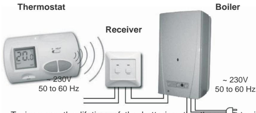
To increase the lifetime of the batteries, the thermostat will not transmit signals continuously. It will only send signals to the receiver whenever it should perform a switch.
