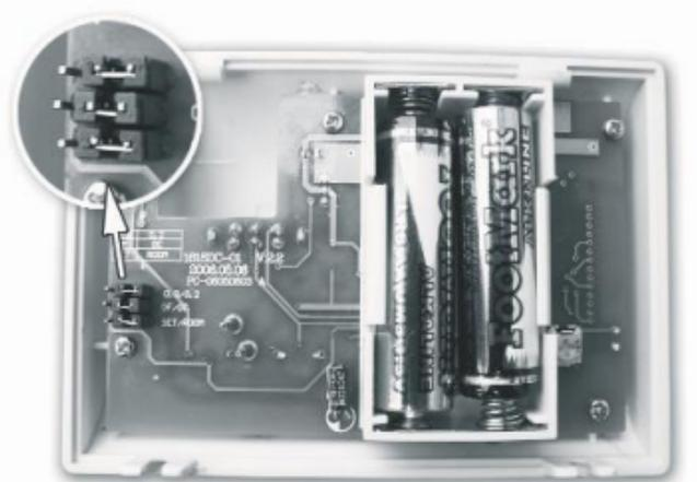
the device is switched on or off) is  $\pm 0.2^{\circ}\text{C}$  that can be modified to  $\pm 0.3^{\circ}\text{C}$  by relocating the plug onto the left and central pins.
