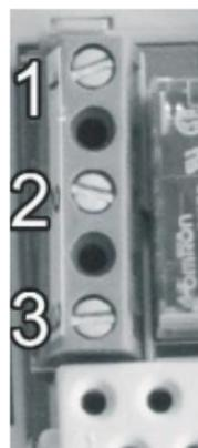
**Attention!** The device must be installed and connected by a qualified professional. Always follow the manufacturer's instructions when connecting the thermostat to any heating or cooling appliance. The voltage appearing at terminal No. **1**, No. **2** or No. **3** depends only on the system being controlled, therefore the dimensions of the wire are determined by the type of the device to be controlled. The length of the wire is of no significance.
